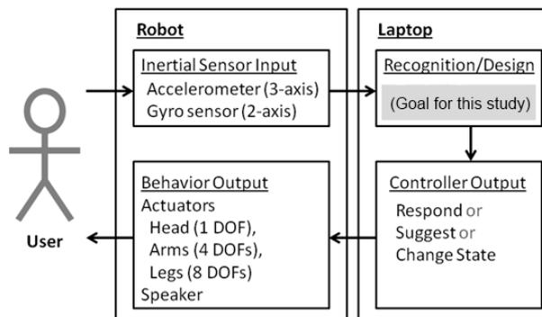
Fig. 3. System architecture: showing the goal of the current study in relation to process flow during a playful interaction.
