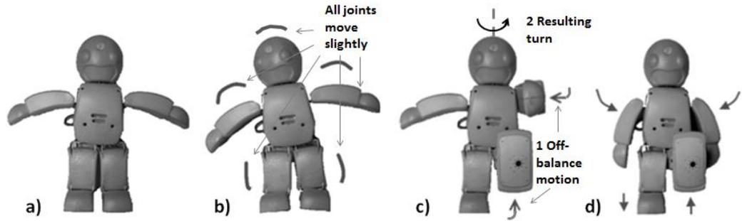
Fig. 5. The four motion conditions investigated: a) No motion, b) Idling (all joints are perturbed by Gaussian noise), c) Try to turn (a sudden motion of the robot’s left arm and leg cause the robot to lose balance and fall to its left), d) Flap arms and legs
