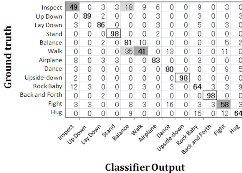
Fig. 6. Confusion matrix for recognizing the 13 target gestures: the three highest true positive scores are shown in outlined cells, the three lowest accuracy scores are shown darkly highlighted, and the greatest sources of confusion are shown lightly highlighted
