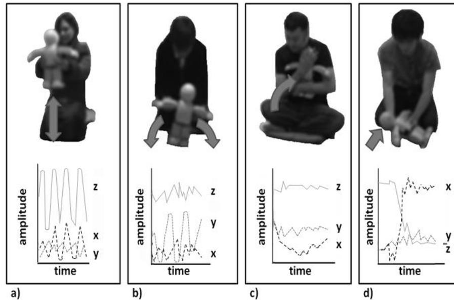
Fig. 4. Gestures being performed (top), with inertial data (below): a) Up Down, b) Dance, c) Hug, d) Lay Down; accelerometer x axis is dark and dashed, y axis is medium shaded and dotted, z axis is light and solid lined
