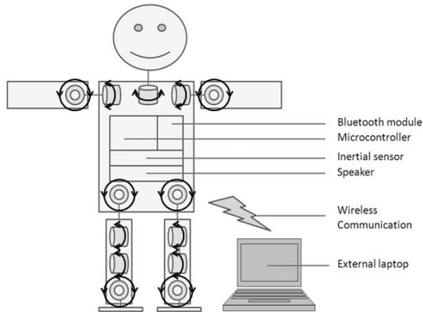
Fig. 2. Sponge Robot’s hardware: degrees of freedom (DOFs) are represented as cylinders with curved arrows indicating the directions of rotation; and the location of components such as the inertial sensor and speaker are indicated.
